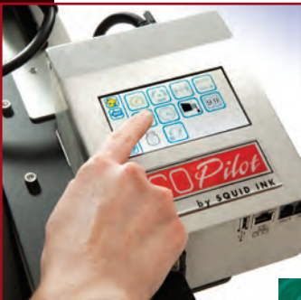
CoPilot's 4.3" full color touchscreen provides access to the systems internal messages and print functions.
