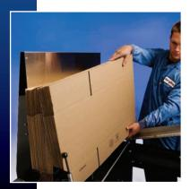
Easy to load input hopper holds up to 90 flat single wall cases and can be loaded by a single person.
