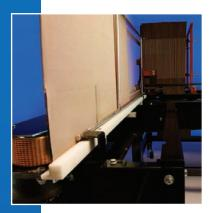
Industrial strength drive belts move boxes consistently through at 72 feet/per min.
