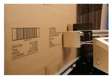
Designed for use with Industrial Ink Jet Printers. Allows printing on all four panels of the case.
